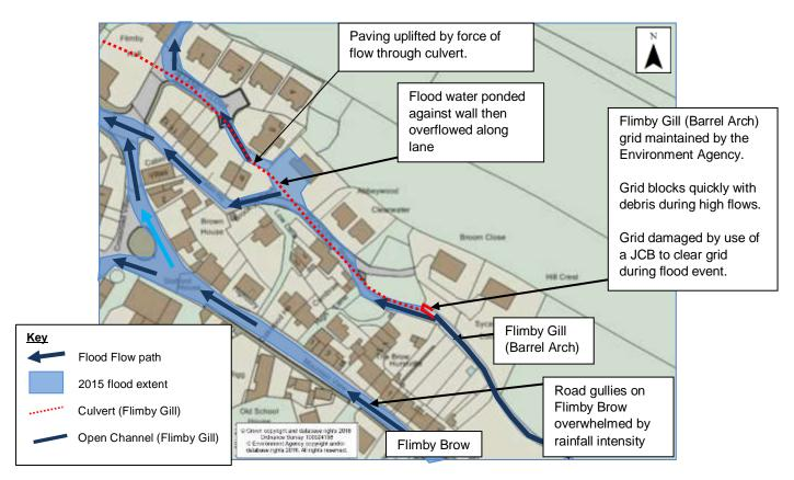
Figure 9: Flimby Gill and Flimby Brow flooding mechanisms
