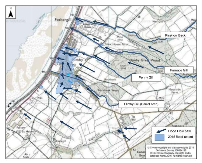
Figure 8: Summary of flood flow routes through Flimby
