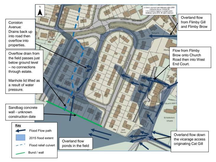
Figure 12: Elm / Coniston / Grange / Solway Avenue and Church Road / West End Close mechanisms
