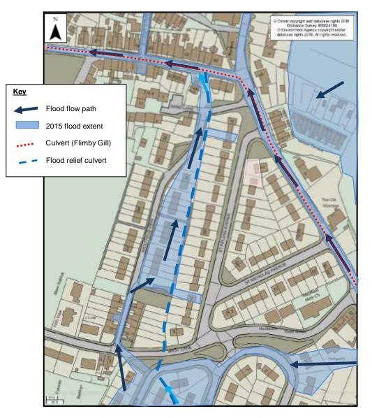
Figure 15: Westfield View Flooding Mechanisms
