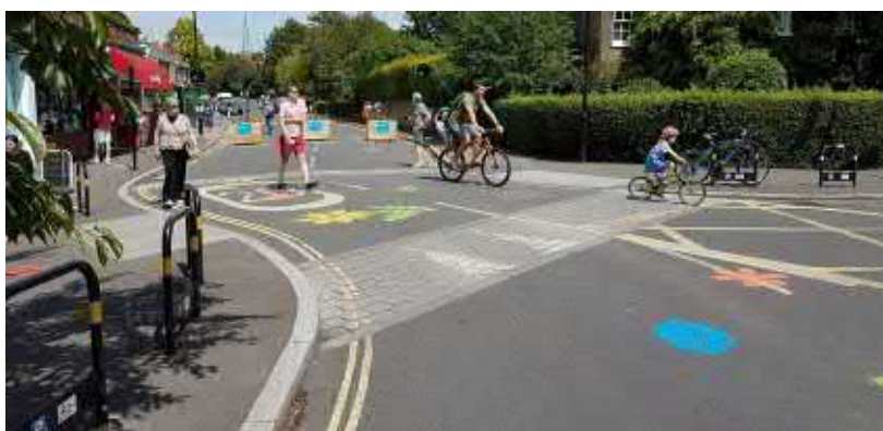
Figure 3.10. Modal filter / LTN
