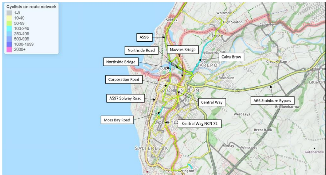
Figure 3-1 - PCT Output: Forecast Cycle Flows Mapped to Route Network, Based on Government Target Scenario
